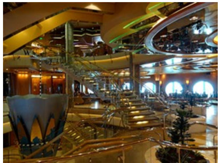
Above right, the extensive use of glass and mirrors is due to the ease of cleaning and their fireproof characteristics.
