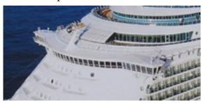
the ship. The bridge dates to the 19<sup>th</sup> century side-wheel ocean-going steam-powered vessels, which had a paddle wheel on each side of the ship. To see the paddle wheels and the sides of the ship, a platform was built that extended outward, like wings, sticking out from the ship for improved vision. It literally "bridged" both sides of the ship, leading to its name.
